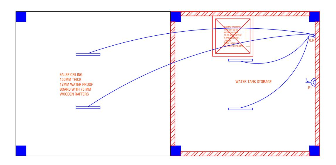
Jamthog Fitting and fixture with wiring layout
