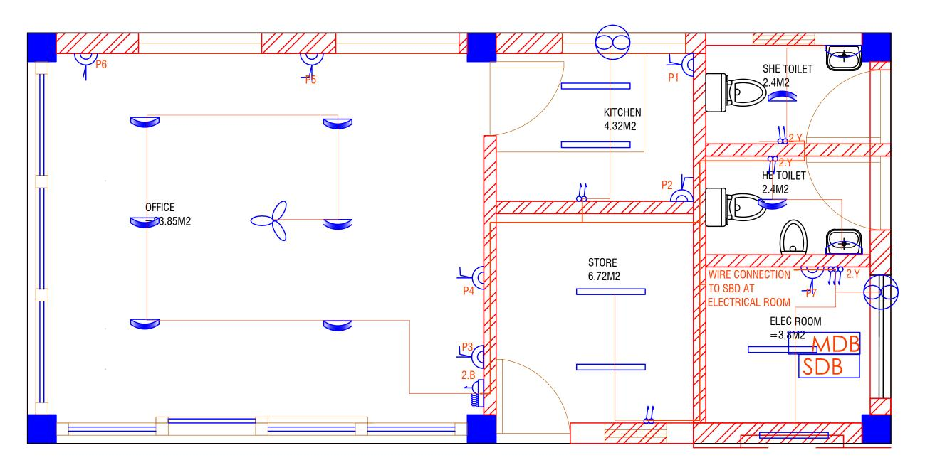
**Ground Floor Fitting and fixture with conduit layout**
