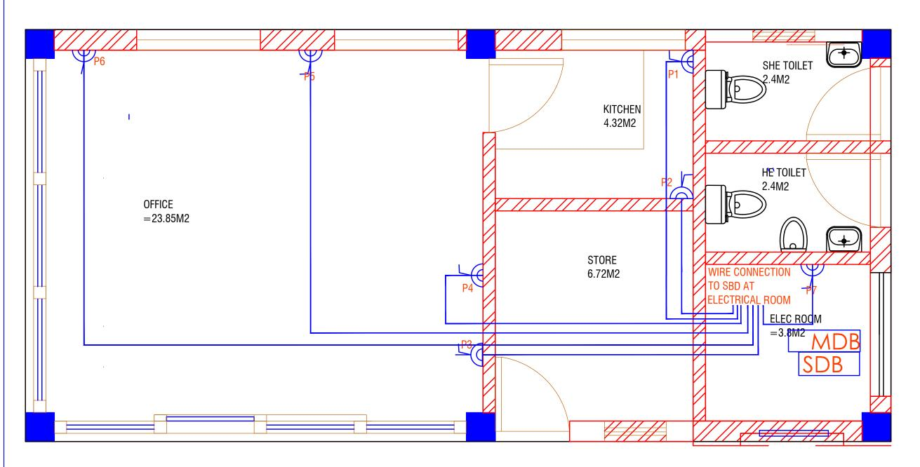
**Ground Floor power point with conduit layout**
